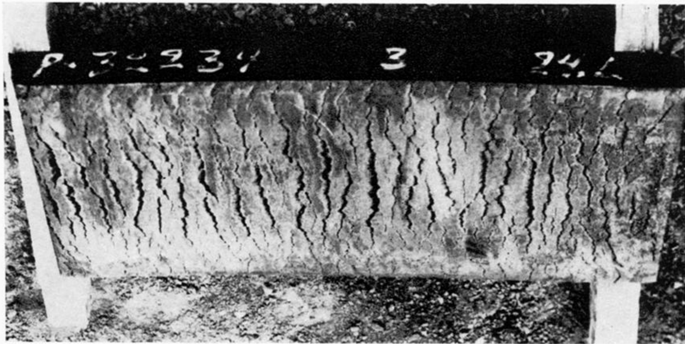
FIGURE 3. Bulk hot shortness in type 316 stainless steel attributed to the presence of 0.0005 % bismuth (by mass) (reproduced from Jensfelt & Norrman 1962).
